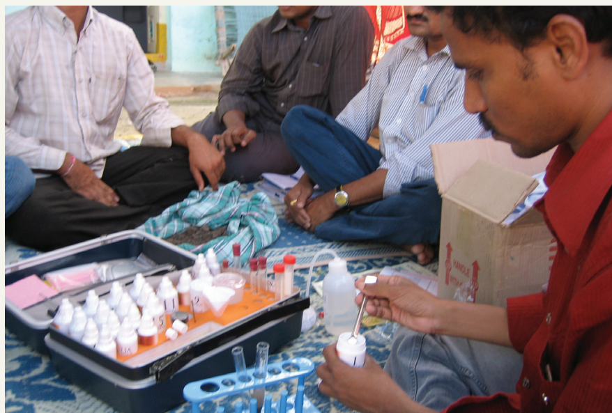
Soil testing kit being used for field soil testing
